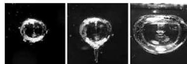
**Figure 3:** Observations of 3 distinct micro-jet types: (left) weak jet ( $\zeta < 10$ ); (middle) intermediate jet ( $\zeta = 0.01$ ); and (right) strong jet ( $\zeta = 0.64$ ) (Supponen et al. 2016)
