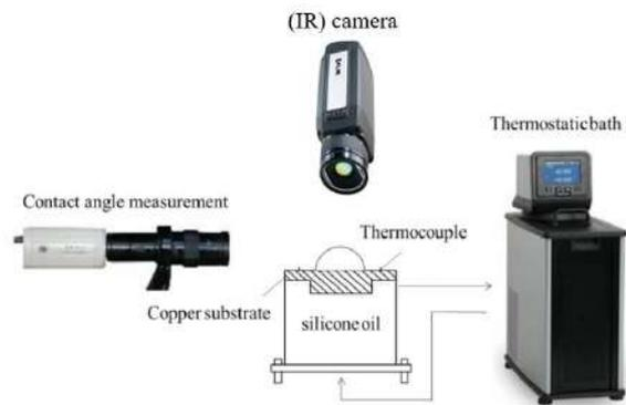
**Figure 1:** Schematic of the experimental apparatus.
