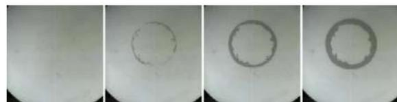
**Figure 2:** Development of the air pocket at disk impact onto a free surface. The data were obtained at  $R_s = 80 \text{ cm}$ ,  $W = 11.1 \text{ cm s}^{-1}$  and the frame rate 2000 fps.
