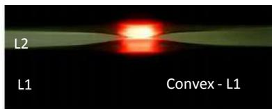
**Figure 3:** A side-view image of the thermocapillary rupture in the Glycerol/Silicon oil pair.
