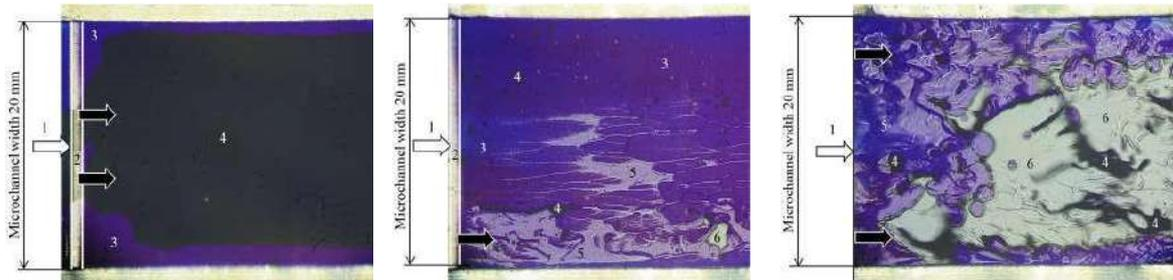
**Figure 1:** Characteristic images obtained by a modified schlieren-method. (a) liquid flow in the microchannel; (b) the formation of the film on the lower wall of the microchannel; (c) the formation of the film on the upper wall of the microchannel.
